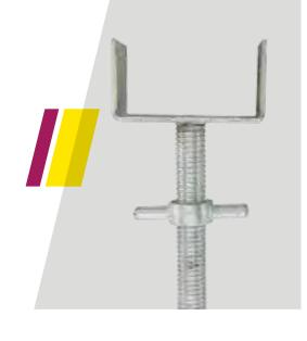
The 'Adjustable' U head offers a 500mm rolled threaded tube which can be adjusted by the wing nut collar. SWL = 4 Tonnes (Concentric Loading)
